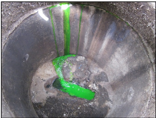
Positive Dye Test (FM-08) 245B
